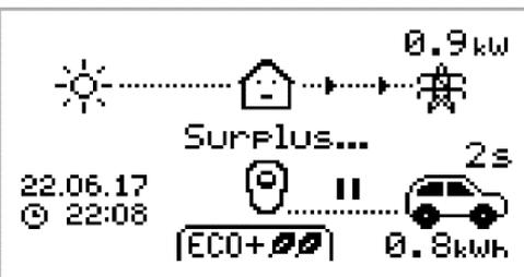
Enough surplus is available and zappi is about to charge the EV. A timer is decremented and can be set in the charge settings (ECO+ mode only).
