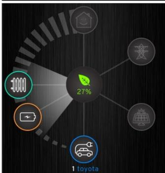
For surplus generation energy, eddi and libbi are of equal highest priority so they will receive any surplus energy equally first. Surplus energy will lastly be offered to zappi which is lowest priority. Although eddi and libbi are of equal priority, because the libbi is positioned below the eddi, libbi can provide energy to eddi. However, libbi cannot provide energy to zappi because zappi is positioned below libbi.
