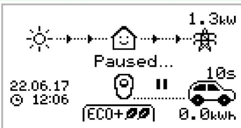
zappi is paused for a few seconds in order to limit the start/stop frequency during ECO+ mode charging.
