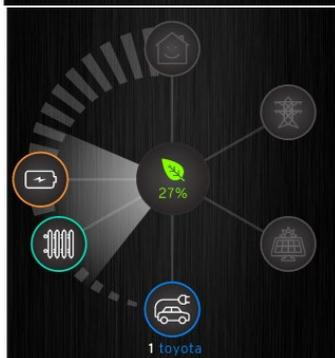
For surplus generation energy, libbi and eddi are of equal highest priority so they will receive any surplus energy equally first. Surplus energy will lastly be offered to zappi which is lowest priority. Although libbi and eddi are of equal priority, because the eddi is positioned below the libbi, libbi cannot provide energy to eddi. libbi also cannot provide energy to zappi because zappi is positioned below libbi. However, libbi can still provide energy to the home.
