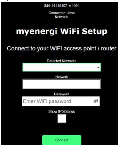
The image shows a black screen with white text for the 'myenergi WiFi Setup' interface. At the top, it says 'myenergi WiFi Setup' and 'Connect to your WiFi access point / router'. Below this, there are several input fields: 'Detected Networks' with a dropdown arrow, 'Network' with a text box, 'Password' with a text box and a lock icon, and 'Show IP Settings' with a checkbox. At the bottom, there is a green 'Connect' button.
