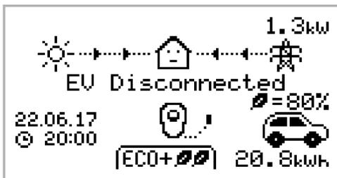
The EV is not connected to zappi.
