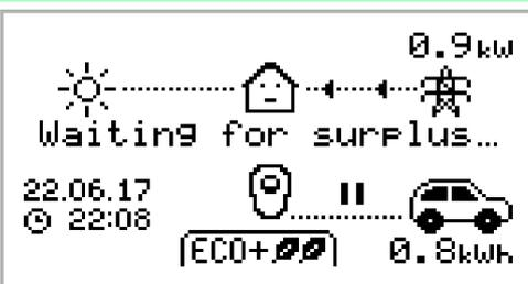
zappi is waiting for sufficient surplus power from the microgeneration system. This screen will be shown in ECO+ mode as it is only in this mode that charging will stop if there is not enough surplus power.
