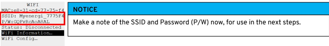
**Step 3:** Connect your smartphone or computer to the myenergi access point by entering your phone or computer WiFi Settings and searching for the network displayed with the same name as the SSID you noted down above. Once displayed, select the network to connect.
