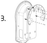
If installing a tethered zoppi you will need to fit the enclosed cable wall guard to the unit using the 4x 4mm x 12mm screws supplied
