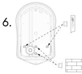
To maintain the IP rating of the unit you must ensure that the bungs provided are inserted in any mounting holes that are not used.
