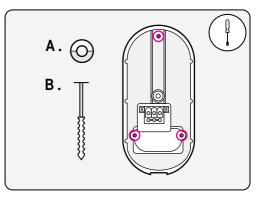
Ensure that the supply cable meets the requirements of the local wiring regulations. Strip cable length of 12mm. Then torque 1.2 to 1.5Nm on each screw.
