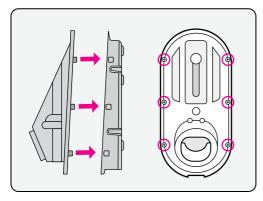
11. Refit the enclosure assembly ensuring clips on both sides make a positive fit to the back box.
