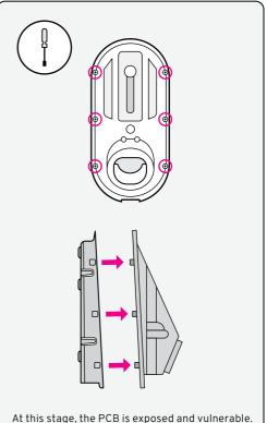
At this stage, the PCB is exposed and vulnerable. Handle with care and place it safely aside to prevent damage, dust, and exposure.
