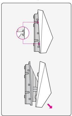
3. Loosen 6X cover screws and remove the front cover assembly from the back box.
