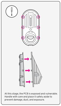
Use the backplate against the mounting surface to mark all the mounting hole locations and then drill mounting holes.
