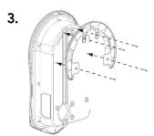
If installing a tethered zoppi you will need to fit the enclosed cable wall guard to the unit using the 4x 4mm x12mm screws supplied.
