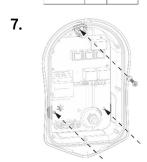
Using the fixing kit provided secure unit to the wall ensuring the sealing washers are used to maintain its IP integrity.
